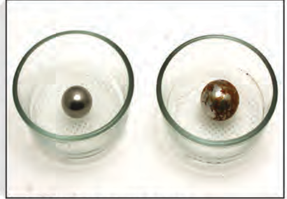
Good and Bad Material Tested in Salt Spray
